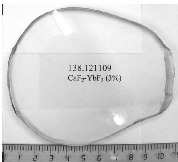
Fig. 1. CaF 2 :Yb (3 mol.% Y) ceramics prepared by deep plastic deformation of its single crystal.
